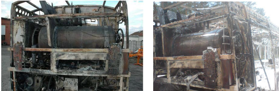
Polish bus fire 2008: only the LNG tanks survived
